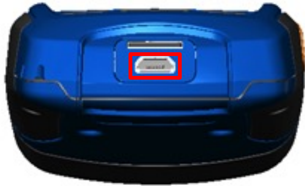
LTO-Quest showing the rear door open and the USB port (for charging) highlighted.
