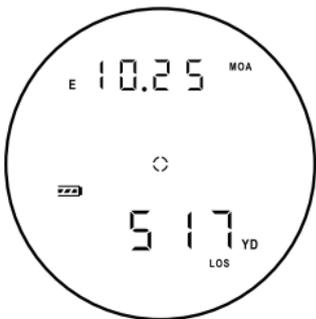
TRIG, a function that is included to support tradesmen and sportsmen alike, displays the true horizontal range and true vertical range, which is based upon trigonometry using angle and line of sight distance. Line of sight distance (LOS) readings will be displayed
