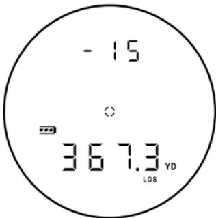
WIND will provide a fixed 10 mph full wind value, meaning it assumes the wind is at 90 degrees to the muzzle. We chose 10 mph as a way for the user to easily calculate corrections on the fly. If the wind is 5 mph, from the 3 o'clock or 9 o'clock position, the shooter would half the hold value. If the wind is 20 mph, the shooter would double the wind hold value. If the wind isn't
