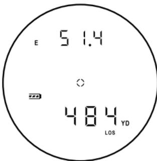
MIL will display the appropriate amount of holdover in milliradians to use, which is based upon the ballistics group and sight-in distance you will choose in a later mode. The lower display shows the line of sight distance to the target. The upper display shows the appropriate number of MIL to hold over or under. In the example to the right, the line of sight distance is
