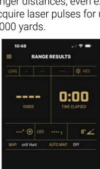
Once the device is locked into the saddle, you can range a target by pressing Remote Fire on the Range Results page. Although you can activate the rangefinder by pressing and holding down the power button, using the Remote Fire button in the Leupold Control App will further enhance stability.
