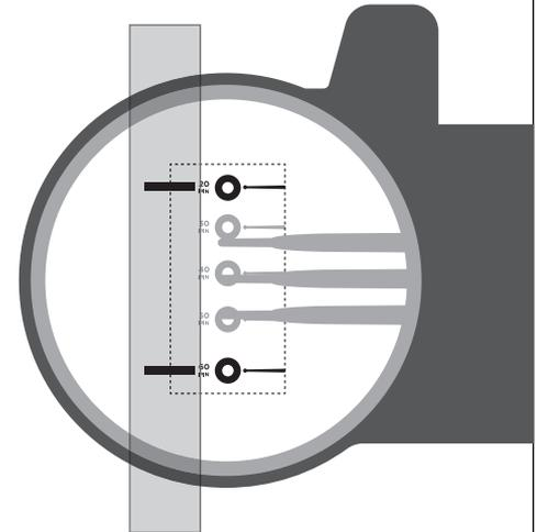
Safely draw your bow, then move forward or backward until your 20- and 60-yard pins align with the 20- and 60-yard pins on this calibration sheet.
