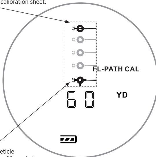
Align reticle with the 60-yard pin at the bottom of this calibration sheet
