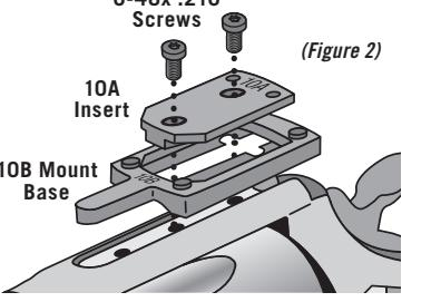
Place the DeltaPoint Pro on the mount base so that the four holes in the bottom of the DeltaPoint Pro will align with the four short posts on the mount base. Then secure the sight with the two M4x.7x15.8mm screws using 25 in-lbs of torque.
